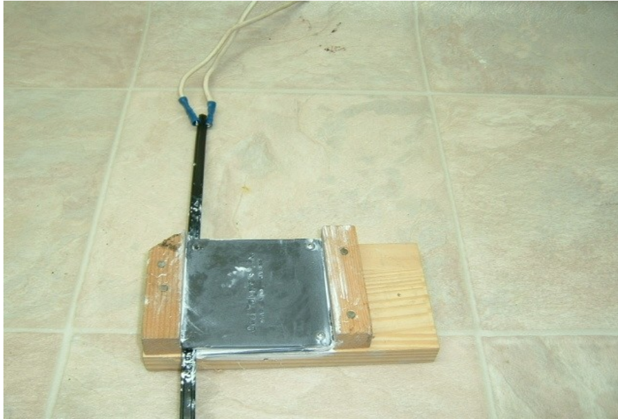
Figure 5.33: Measurement of heat spread on a thermoplastic plaque at one end.
