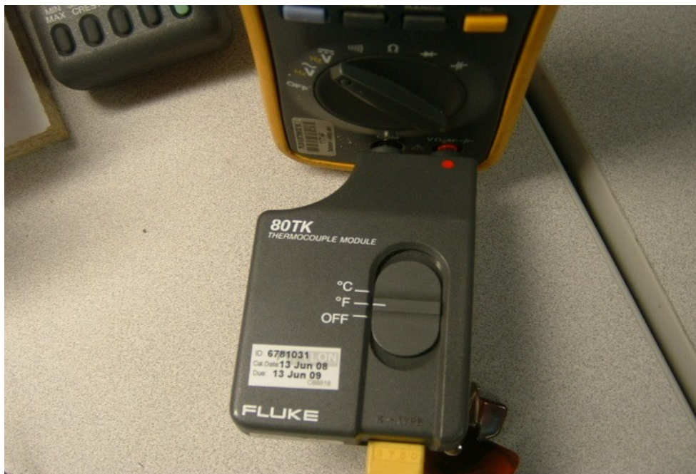
Figure 5.21: Fluke 80TK thermocouple to millivolt convertor.
