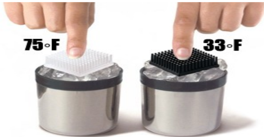
Figure 3.2: Example of temperature measurements with regular plastics and thermally conductive plastics (Source: Cool Polymers).
