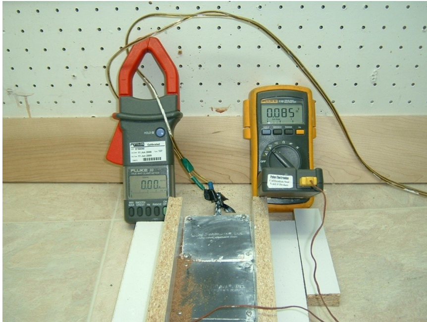
Figure 5.31: Stage- 3 embedded setup and temperature during cooling cycle at 11.01 AM.
