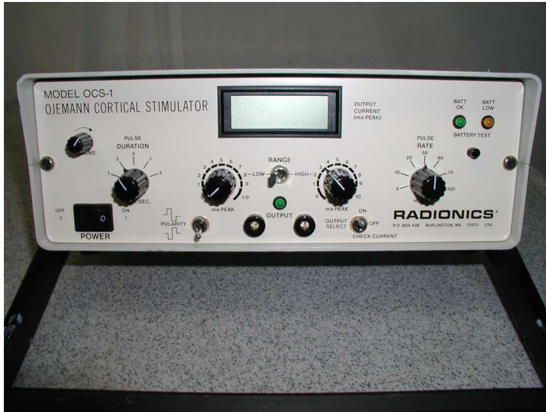
Figure 3.8: Ojemann OCS-1 bipolar stimulator. The Ojemann OCS-1 is capable of peak-to-peak currents of 0-22 mA, in pulses of 0.1-2 ms, at frequencies of 5-100 Hz.
