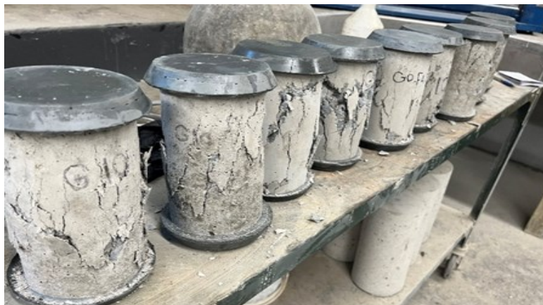
Figure 3-10: Specimens after compressive strength test
