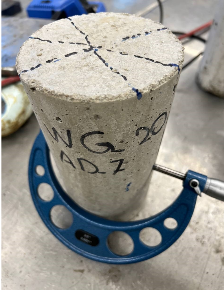
Figure 4-2: All the specimens are centerline marked, and the diameters are measured in three different directions using a caliper.
