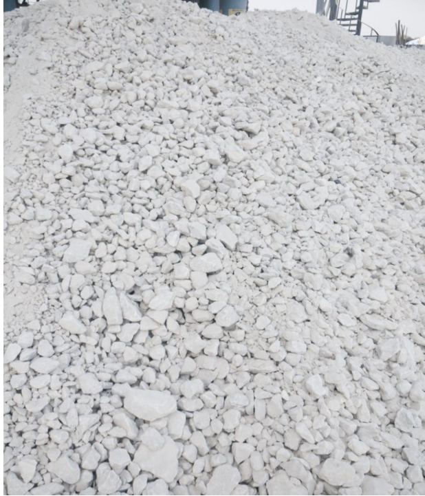
Figure 2-3: Natural gypsum. Source:( https://quarro.in/ )
