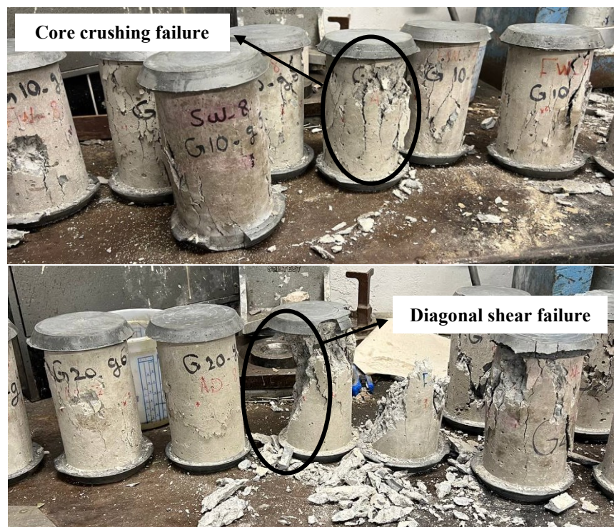
Figure 4-4: Specimen's failure modes after compressive strength test
