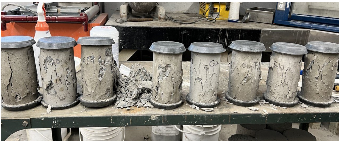
Figure 3-11: Failure modes after compressive strength results
