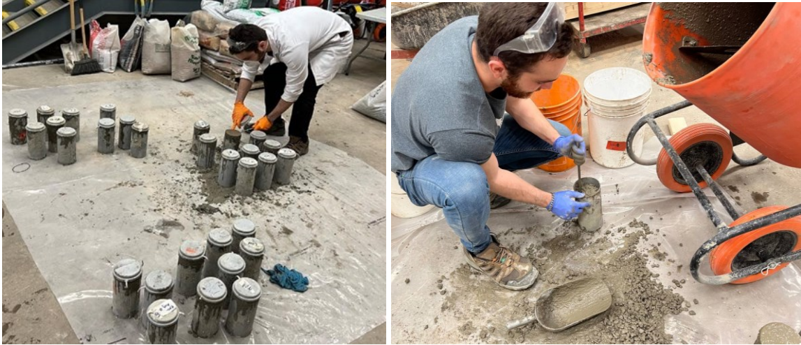
Figure 3-6: Casting concrete in molds and preparing specimens.
