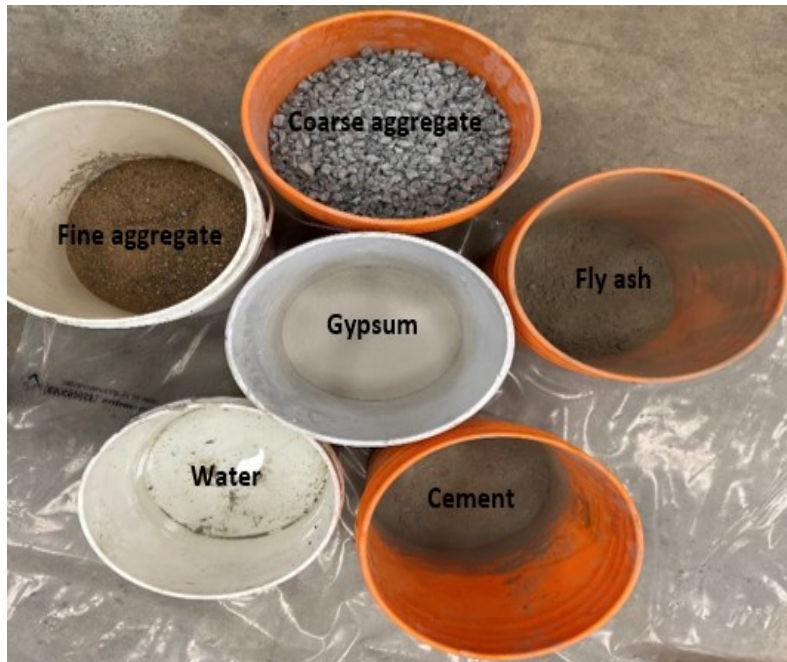
Figure 3-5: Gypsum concrete ingredients
