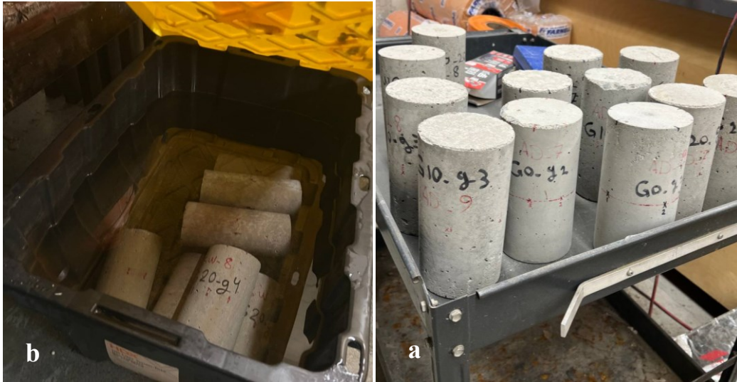
Figure 4-1: a) Specimens exposed to room atmosphere (air dry condition), b) specimens kept in the water containers for wet exposures.
