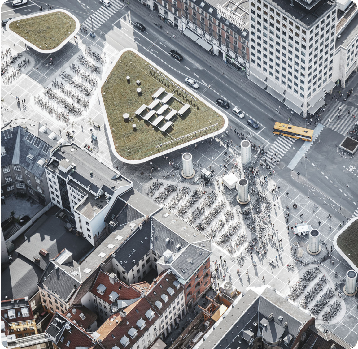
Aerial view of Denmark's busiest train station, renovated in 2015. The station sees over 250,000 passengers daily, with 2,500 bike parking spots sunken 40cm into the pavement to preserve pedestrian sight lines along the linear plaza. (Cobe n.d.)
