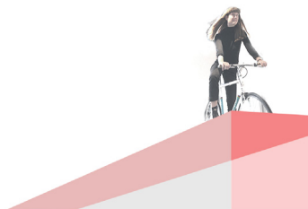
8% slope (1:12) is maximum for stretches under 150m.
