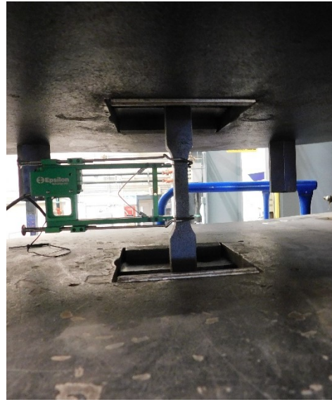
(b) Instron Universal Testing machine set-up
