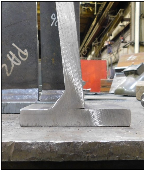
(a) Trial connection with no tack welds or tie bar (b) ETLCC connection with tack welds and tie bar
