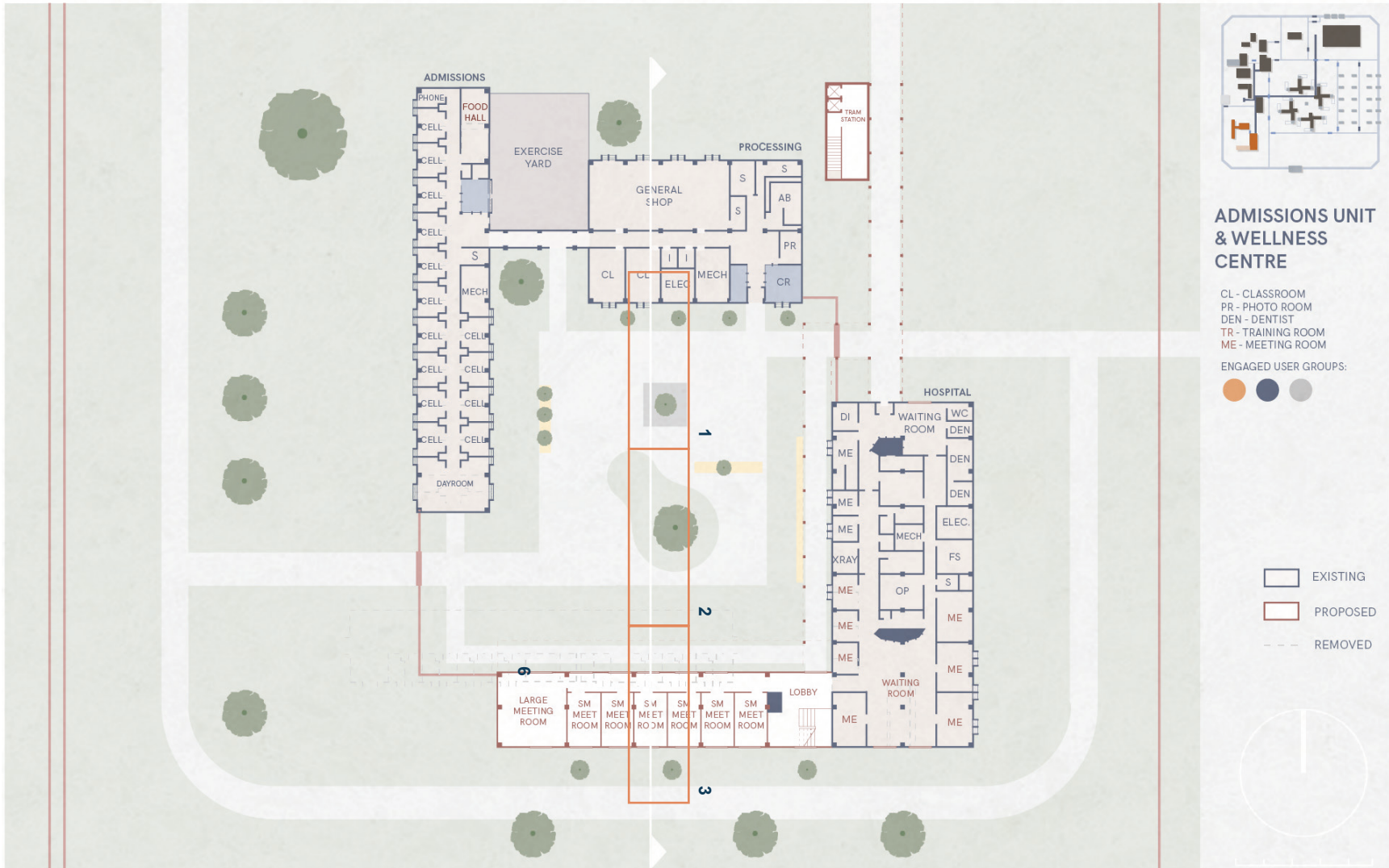
Admissions and Wellness Centre plan, the admissions and hospital wing needs a bit more security so the exterior space is left enclosed (1). Within that, both exterior spaces (2) and interior (3) are considered for different types of support, with a new wing focusing on mental health.
