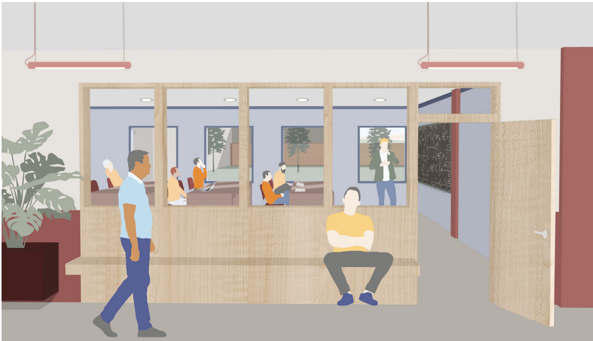
Example of views between programmed and circulation spaces, which increases likelihood of informal surveillance through people passing by.
