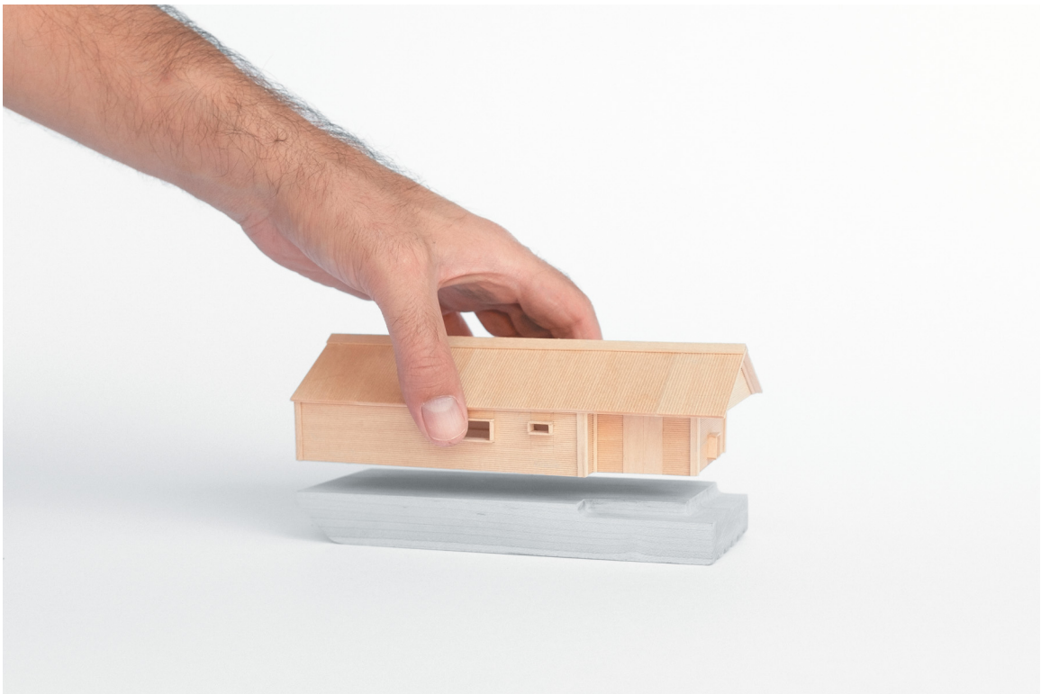
Model: 1/8"=1' (N.T.S. in photograph) illustrating the floating concrete foundation and the light-frame enclosure built on top once the foundation arrives on site.
