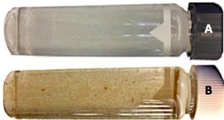
Figure 6.5 Turbidity samples measured from (A) the flowing pipe discharge and (B) the 6-hour stagnation period obtained under the low manganese, 0.7 mg-PO 4 /L experimental condition.
