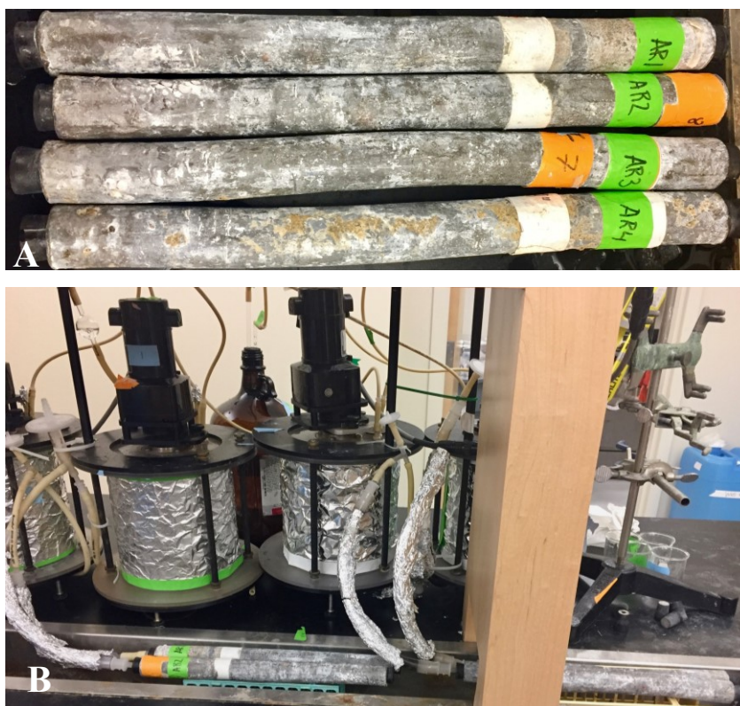
Figure 6.1 The harvested lead-pipe sections (A), and the experimental set-up, with annular reactor discharge being fed into the lead-pipe sections (B).
