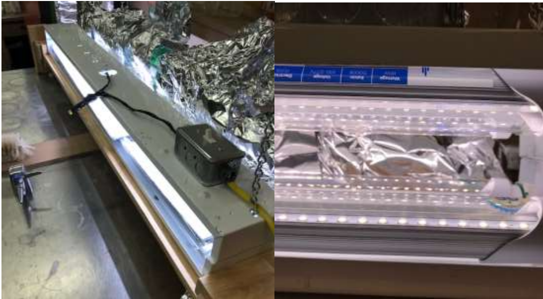
Figure 3.3: High light intensity chamber producing an illuminance of approximately 13,500 lux
