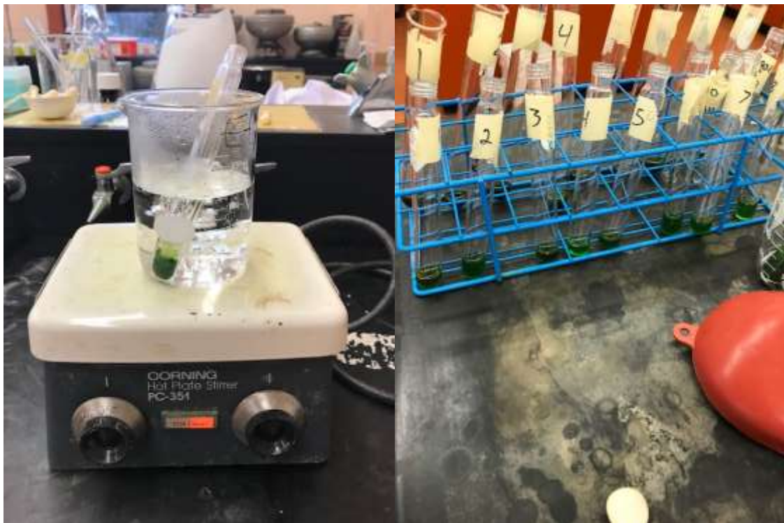
Figure 3.5: Protein extraction process showing how boiling the sample induces the separation (left) as well as the extracted protein-containing top layer (right)
