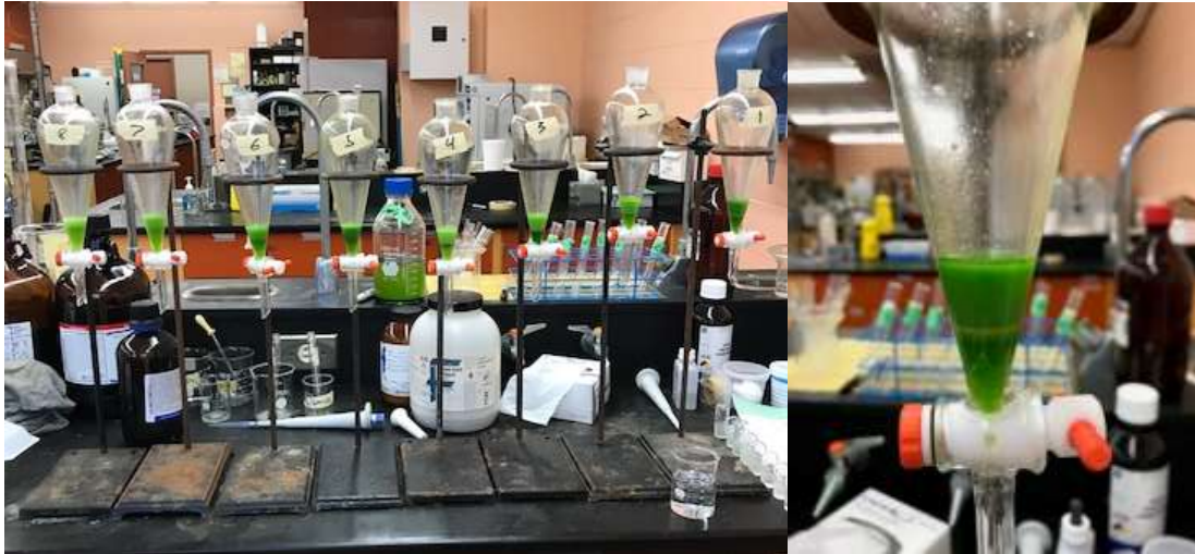
Figure 3.4: Lipid extraction process showing the separation of the lipids from the algae biomass
