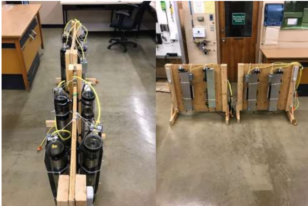
Figure 3.7: Front and side angles of the completed photobioreactor systems
