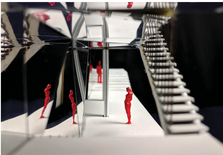
Model photos of early horizontal circulation core design experimenting with a mirrored material rather than black oxidized steel.
