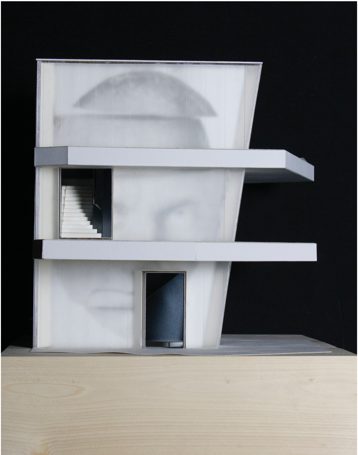
Model photo of circulation core with interior perforated image appearing through the translucent polycarbonate exterior cladding during day.
