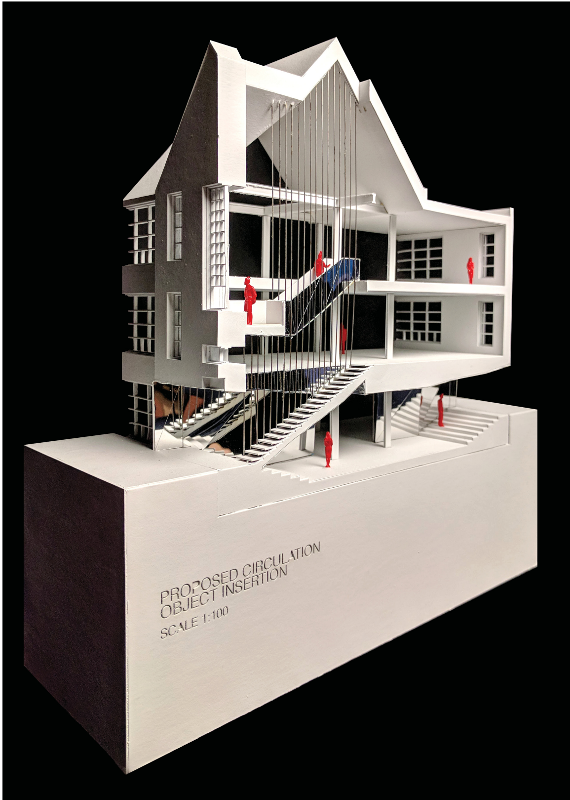
Section model [1:100] photo of horizontal circulation core between the courtyard and former bus slips.
