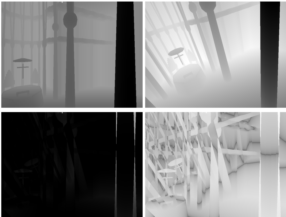
Figure 4.8: Depth image of target B (top left), a candidate depth image (top right) and the images obtained by computing pixel-wise differences with different power value P = 2.0 (bottom left) and P = 0.1 (bottom right; both with intensities normalized).
