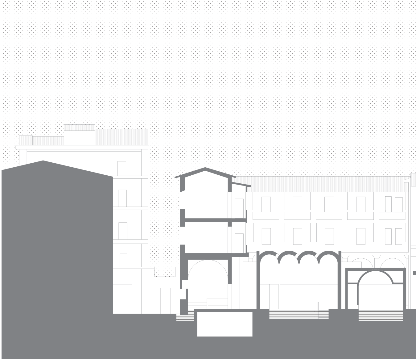
Section cutting through the three courtyards
