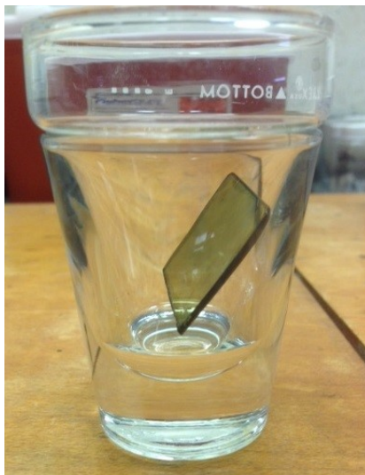
Figure J2. A photograph of a D1-A1 thin film undergoing SVA in an annealing chamber.
