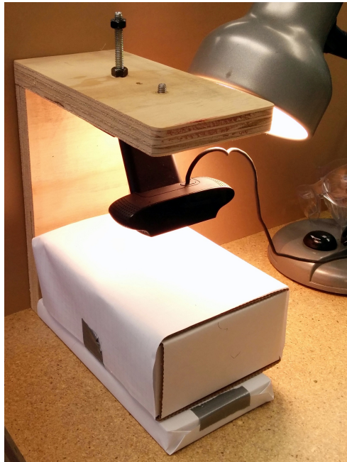
Figure 5.1: Setup for precise stent measurement and cataloging
