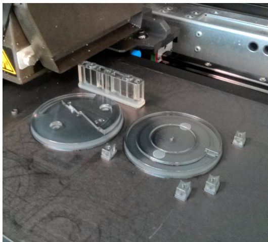
(a) three-dimensional printing of clear wire bending jig
