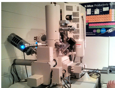
(e) Etch and analyze using the SEM and EDS
