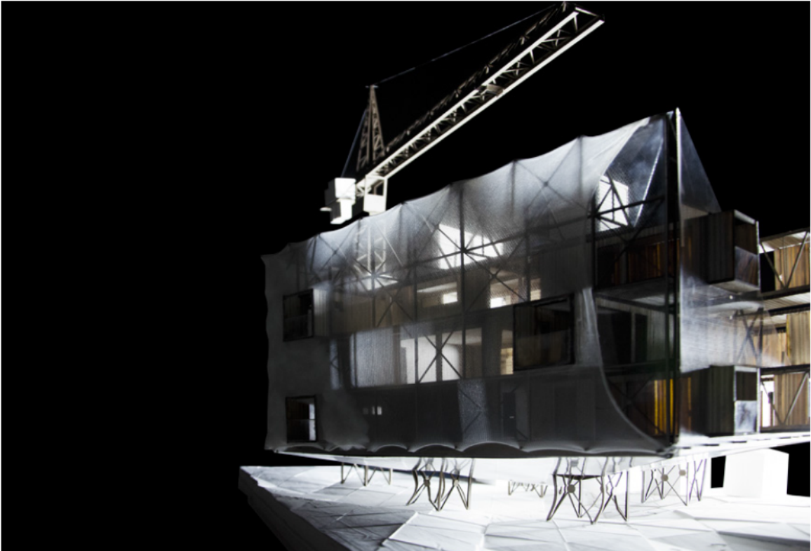
Elevation of building model showing the exterior snow mesh facade as it would appear during the summer.
