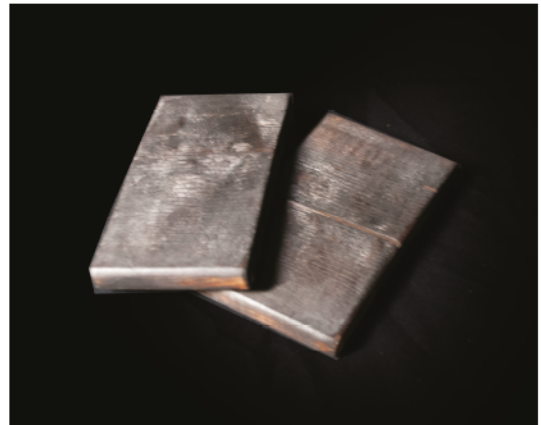
Figure 113: Exploration of carbonized (charred) siding for waterproofing.
