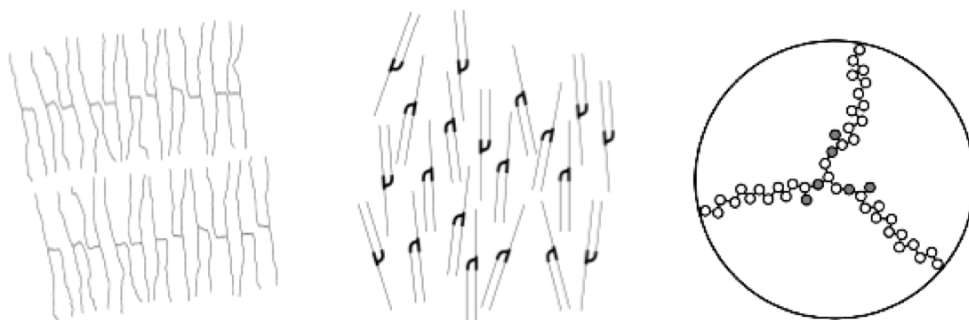
Figure 2-3 a (left) proposed structure of TAGs in liquid by Larsson (1972); b (middle) proposed structure of TAGs in liquid by Cebula et al., (1992); c (right) proposed “Y”-conformation within each “disc”, where TAG fatty acid chains spread out at \sim 120^\circ to each other in a single, though diffuse, plane (Corkery et al., 2007).
