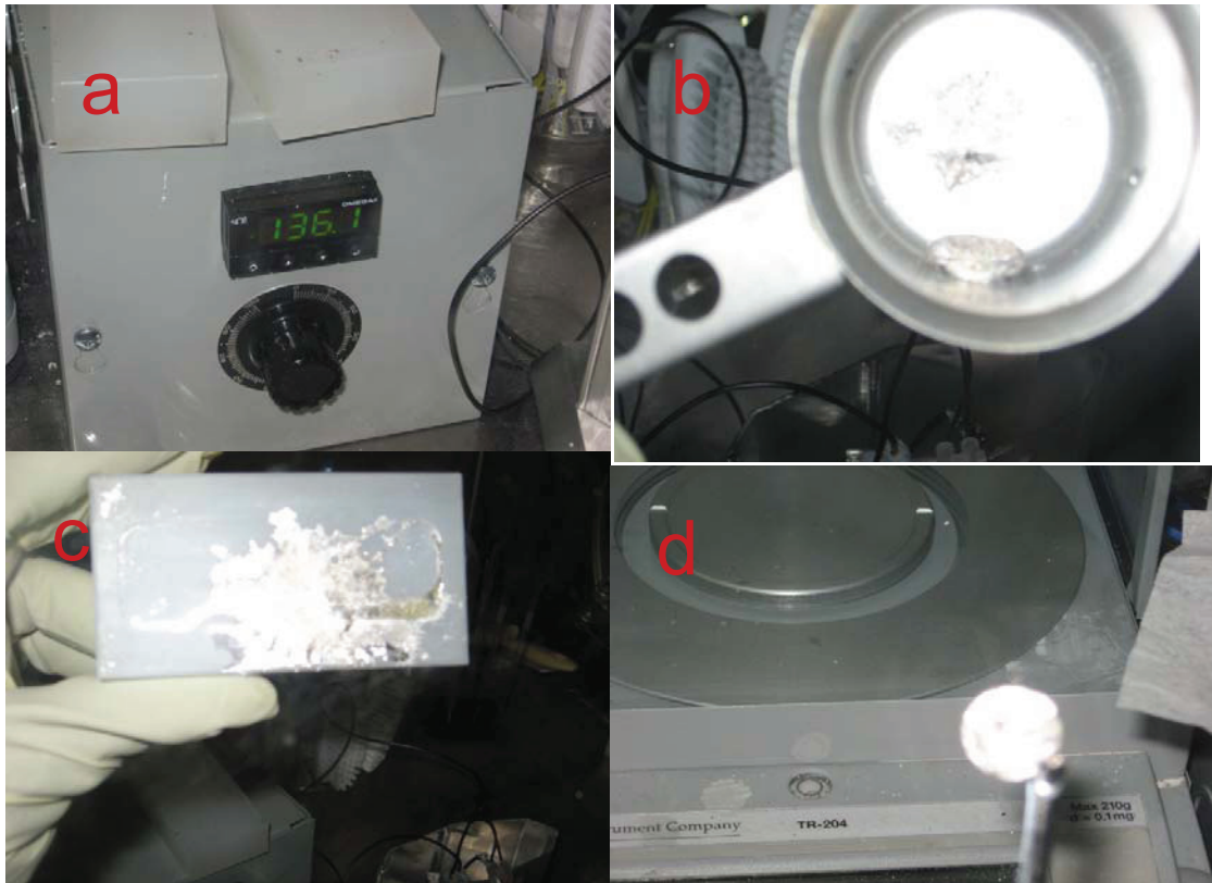
Figure 2.3 Process of making sodium foil. a). A home-made temperature-controlled furnace; b). Liquid (molten) sodium in a stainless vessel; c) a piece of sodium foil on the polypropylene plate; d) a punched sodium foil that is ready for coin-cell assembling
