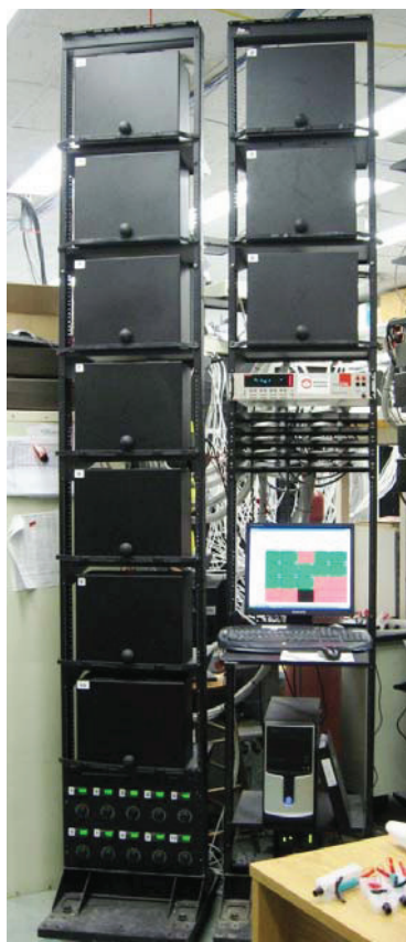
Figure 2.13. A picture of the 190-channel automated cell storage system
