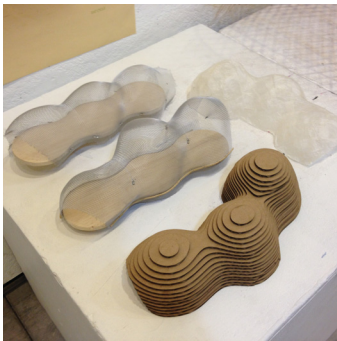
From top left to bottom left: Gridshell jig used to make matt of lathes. Ribs used to create 1:50 model. Some process models with different materials describing form and lightness. Right: Experimenting with different gridshell forms.
