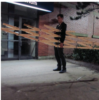
The 1:1 shell detail with double layer construction. Here is an example of what can be possible with pin connections and scissoring.
