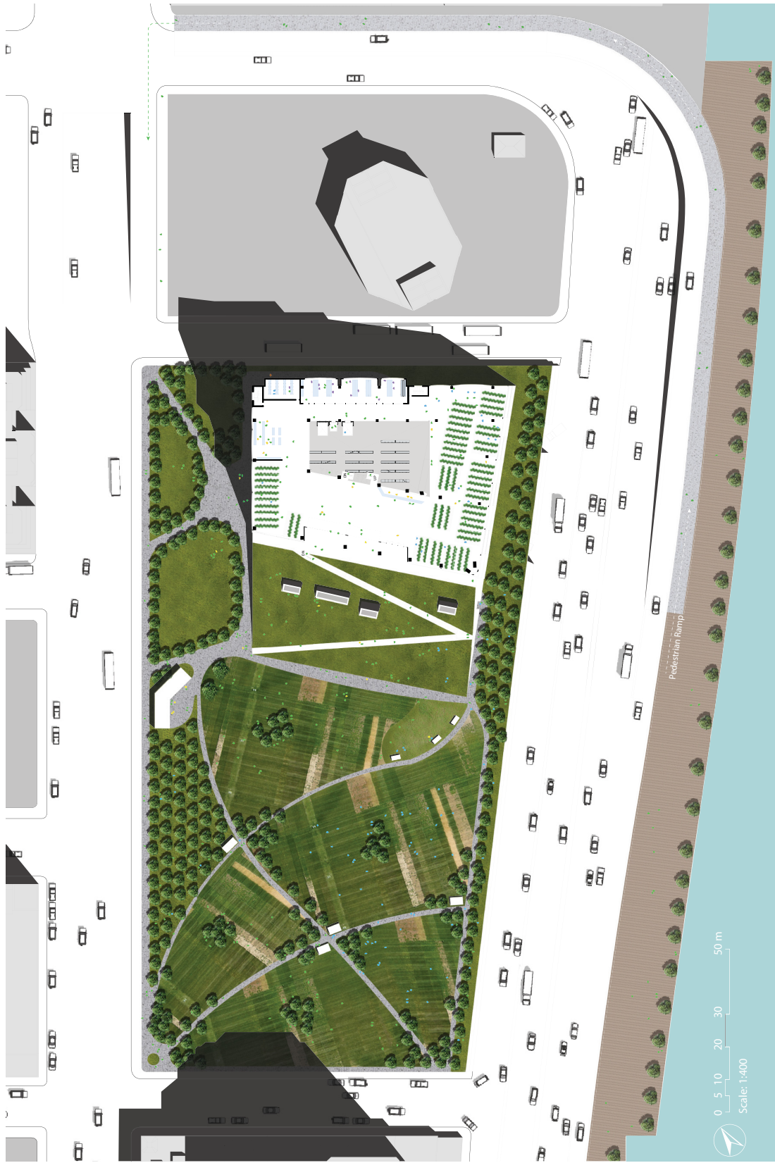
Figure 2.12: Overall site plan showing the extended waterfront esplanade with the new pedestrian ramp.
