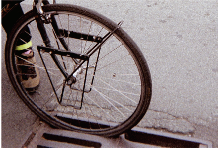
Figure 4. Tire getting caught in a storm grate.
