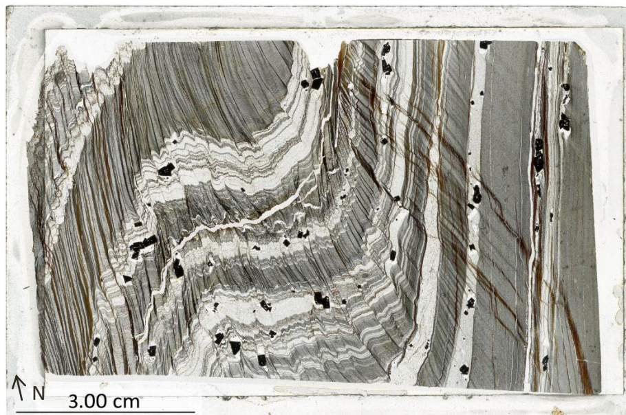
Figure 6.6: S_2 crenulation fabric overprints continuous transposition cleavage ( S_2 with S_0 parallel (sub-vertical in photo)) in Halifax Group slate, southeast boundary of Cape St. Marys Shear Zone (from Culshaw & Liesa, 1997).
