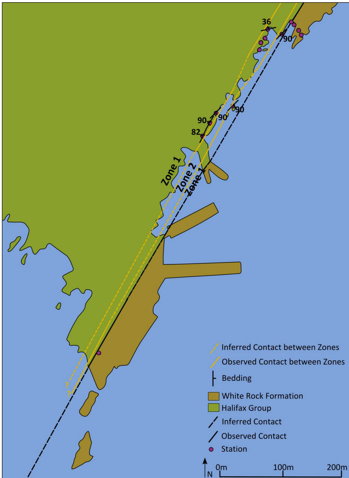
Figure 4.9A: Bedrock geology map showing select bedding measurements observed in the Halifax Group used to define 2 zones observed: Zone 1 - bedding at a high angle (almost parallel to the S_{x2} cleavage fabric) and forming plunging close asymmetric overturned folds; Zone 2 - bedding at a lower angle (further from the S_{x2} cleavage fabric) and forming plunging symmetric folds.
