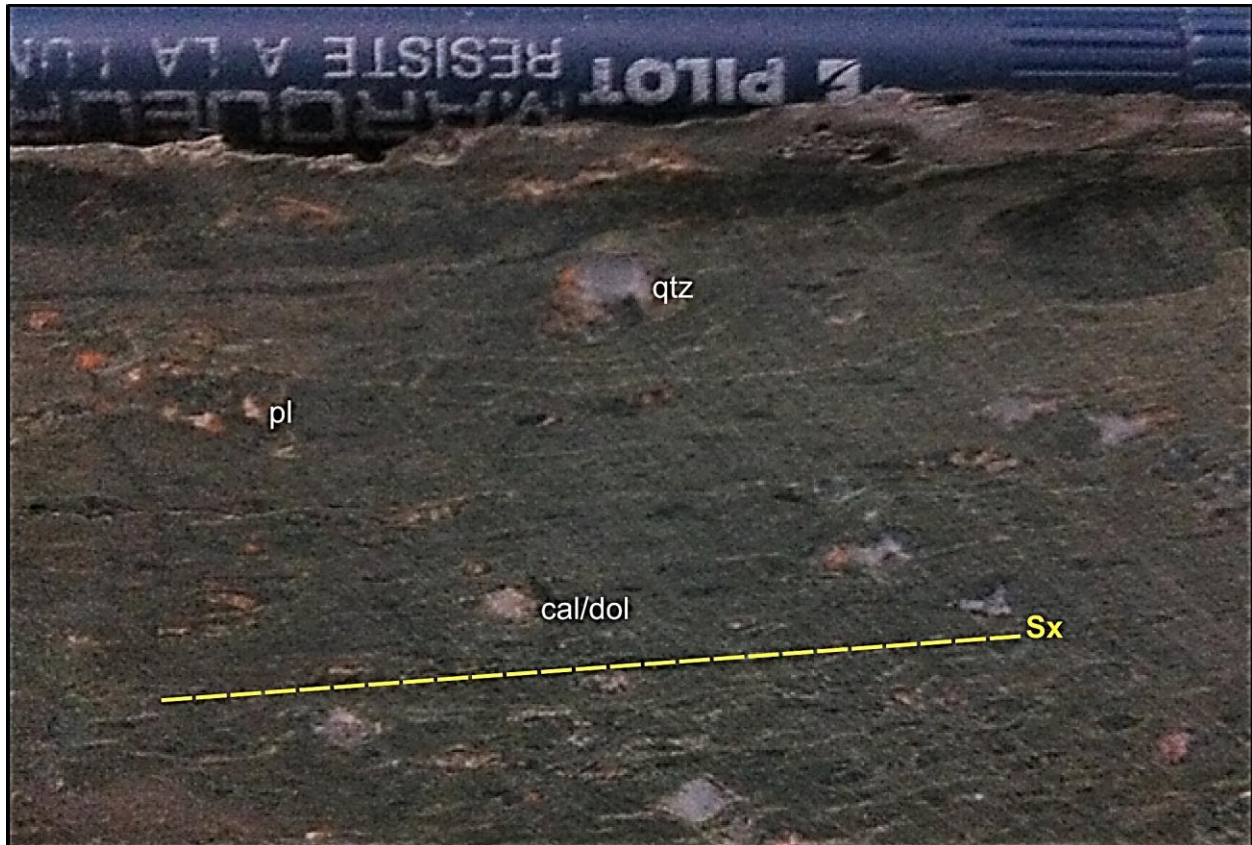
Figure 4.4: Oriented sample from WRF greenschist basalt, cut perpendicular to S_x cleavage surface. Porphyroclasts after phenocrysts of plagioclase and quartz, and calcite vesicles are visible (pen for scale, 6cm) (Station 010).
