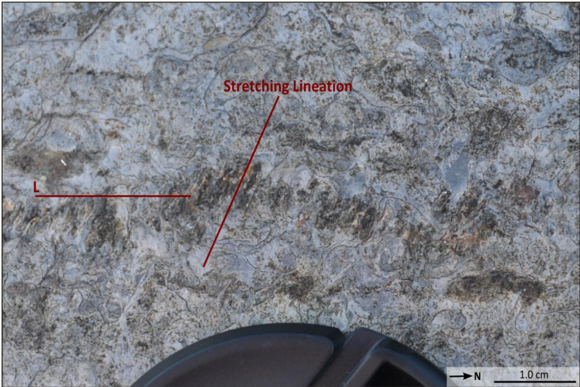
Figure 4.11B: Stretching lineation formed from quartz fringes on pyrites labelled with approximation of visible lineation fabric indicated (Station 008).
