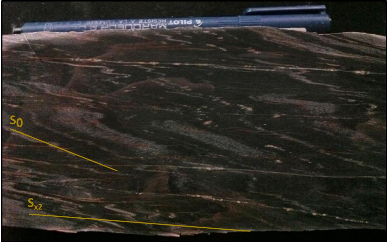
Figure 4.10: Oriented sample cut perpendicular to S_{x2} and S_0 , showing asymmetric folds associated with the first zone in the BRF slate (Sample CD_12_005) (Station 008).
