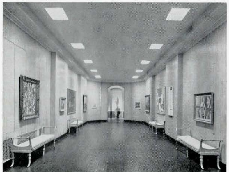
Fig. 5—Reception Room of Chicago Art Institute in the Goodman Theatre, Chicago, Illinois. Wall lighting from reflectors above ceiling panels.
