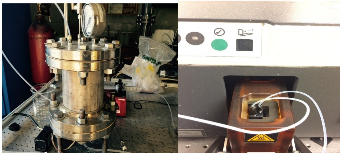
Figure 6-1: Heated water vessel (left), and the flow through cell within the transmission module of the FT-NIR (right).
