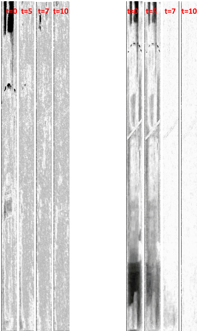
Figure 3-9: Variance normalized images during amine injection into a 1" pipe without (left) and with (right) and orifice plate present ( \beta=0.7 ). Flow is in the upward direction.
