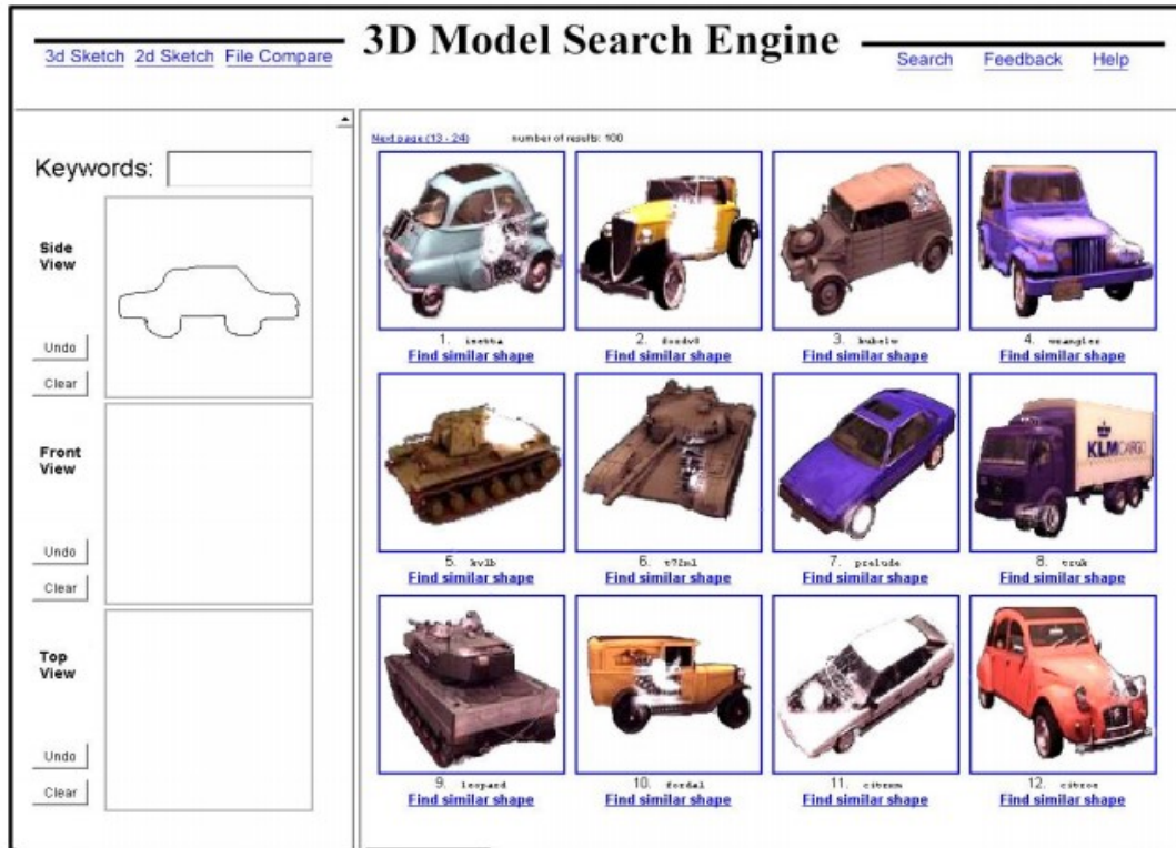
Figure 2.5: The query interface of the 3D search engine proposed by Funkhouser et. al (Funkhouser, et al. , 2003).
