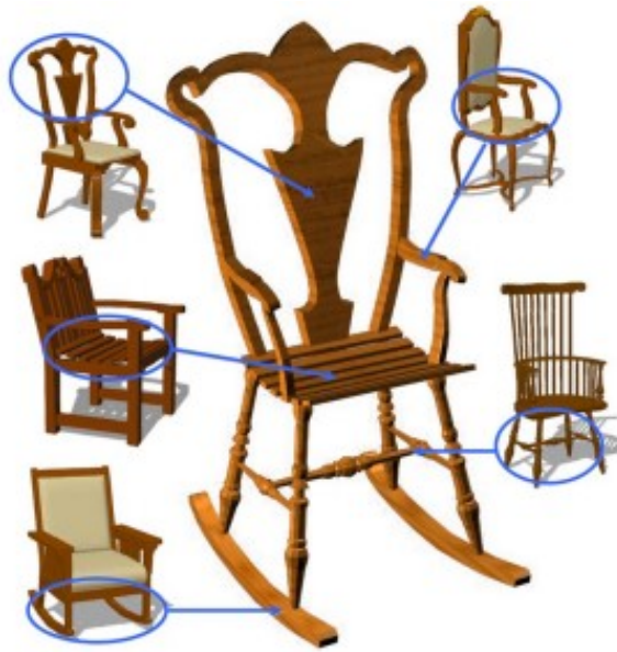
Figure 2.6: An example schema of Modeling by Example (Funkhouser, et al., 2004): The center large brown chair is generated from the circled parts of the other objects.
