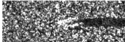
Figure 2.2: Side-scan sonar object (center) with shadow (right).
