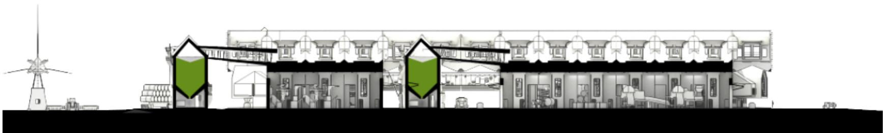
East by West Building Section_Hempworks Decortication Facility_Looking South to Decortication Equipment through the Heated Workshop.
