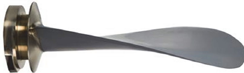
Figure 2-7 Composite propeller blade, attached to the bronze blade interface to existing metallic propeller hub [135].
