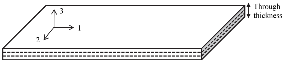
Figure 3-1 Directionality of typical laminate.
