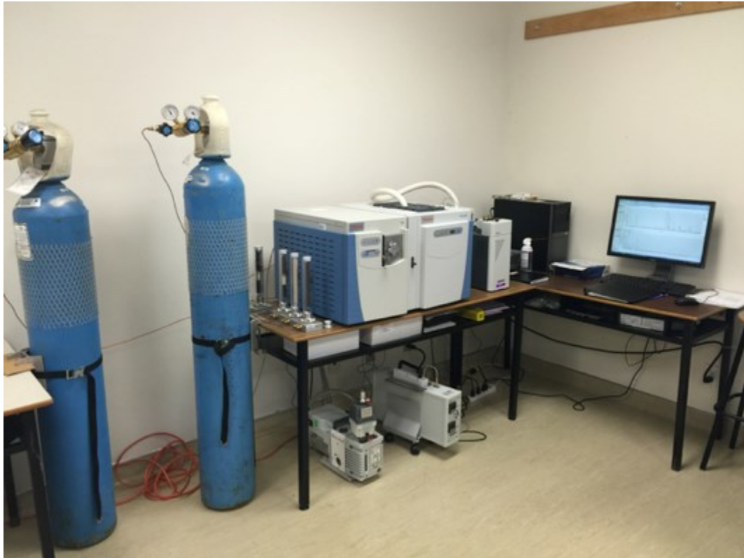
Figure 10. TD-GC-MS system setup showing the nitrogen and helium gas supplies.
