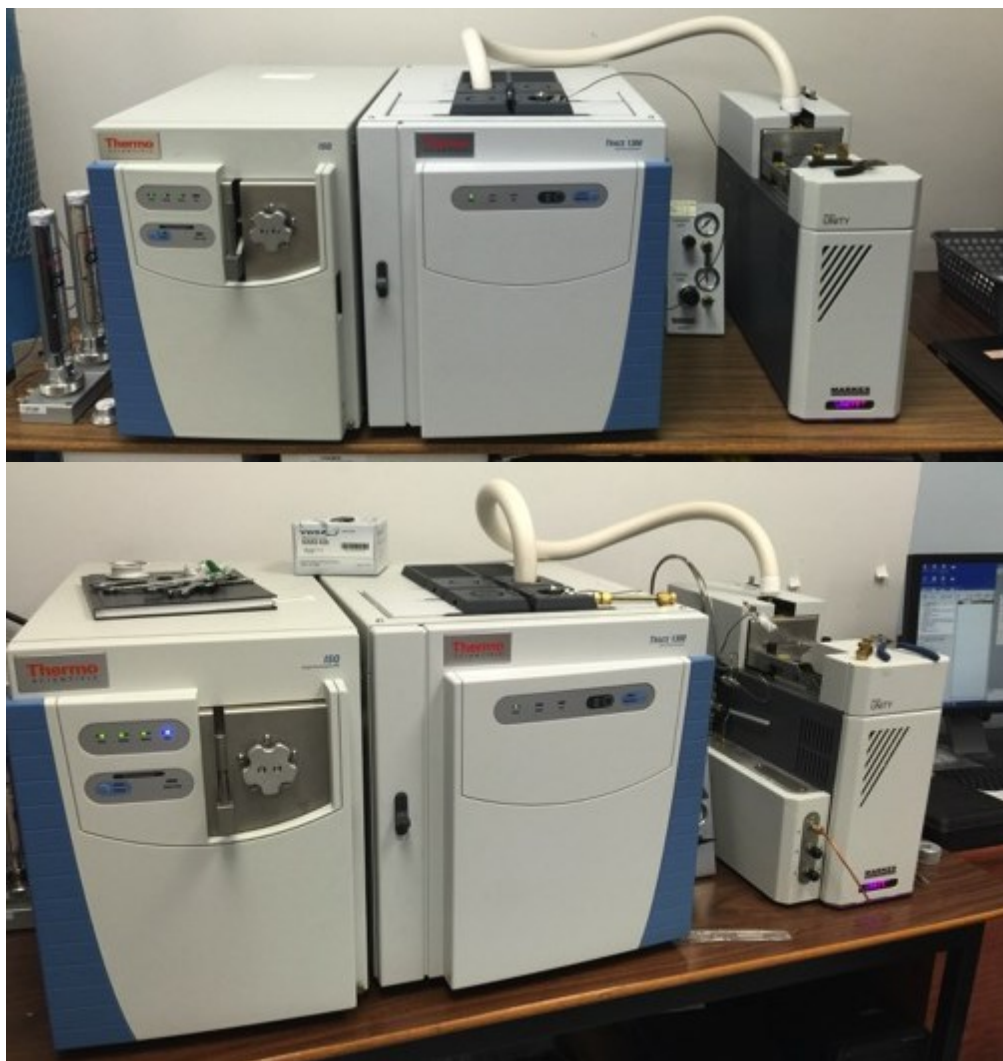
Figure 11. Markes International Unity-2 thermal desorption-Thermo 1300 gas chromatography-Thermo ISQ mass spectrometry systems (TD-GC-MS)
