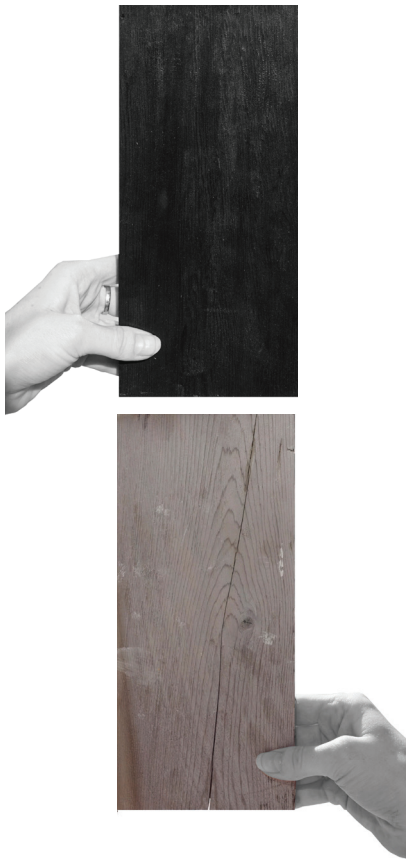
Figure 30. Blackened cedar lath (top), naturally greyed cedar laths (bottom)
