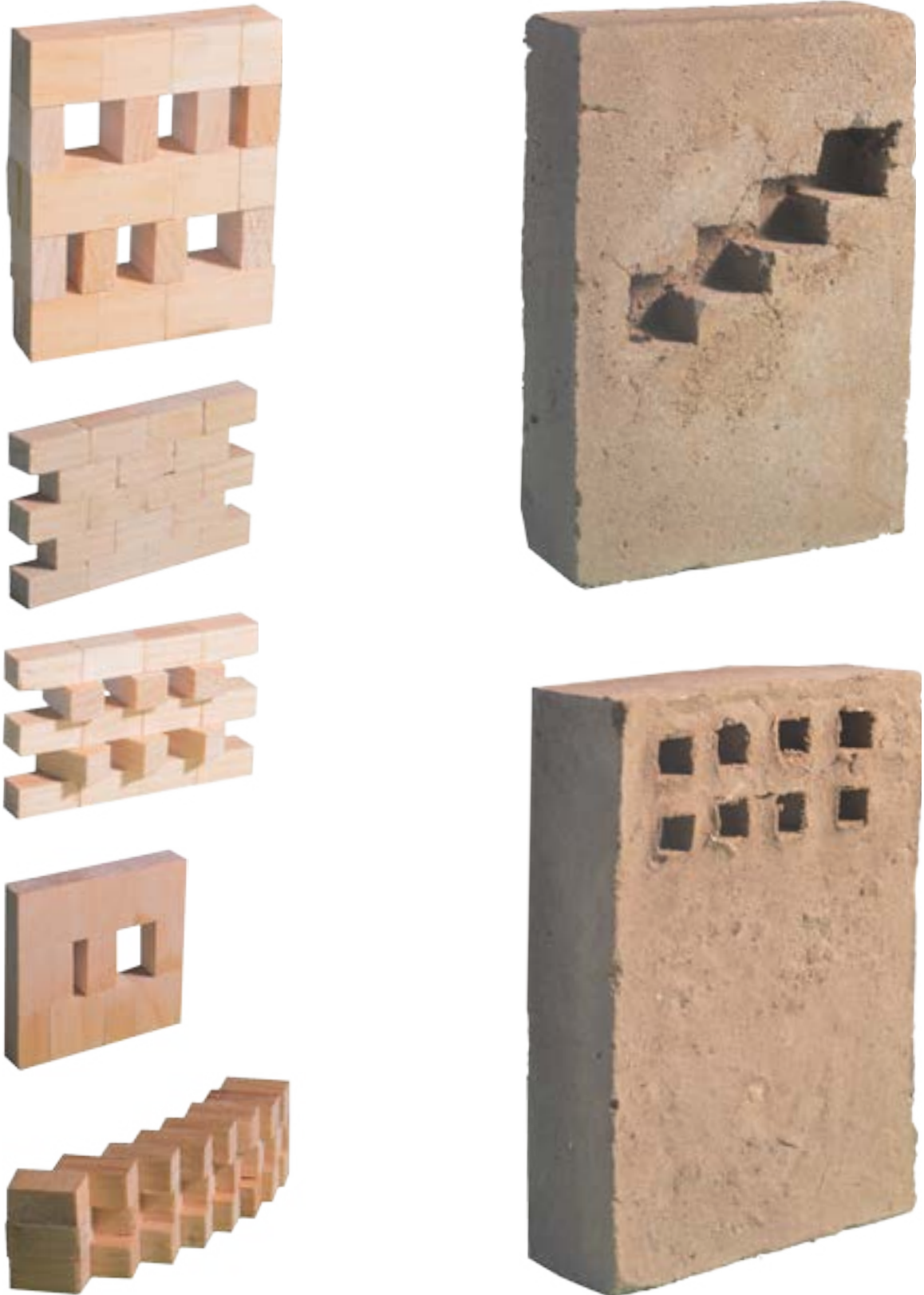
Sketch models exploring different brick stacking arrangements so as to allow for good ventilation (left) and exploring the nature of voids created within brick walls for different reasons such as stairs (top right) and ventilation (bottom right)
