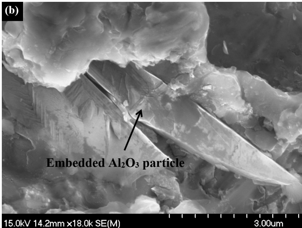
Figure 4-7 SEM micrograph of steel specimen after erosion at 30° impact angle (a) micro-forging of the surface (API X42, 36 m s -1 ) and (b) embedded Al 2 O 3 particle (API X42, 36 m s -1 ).
