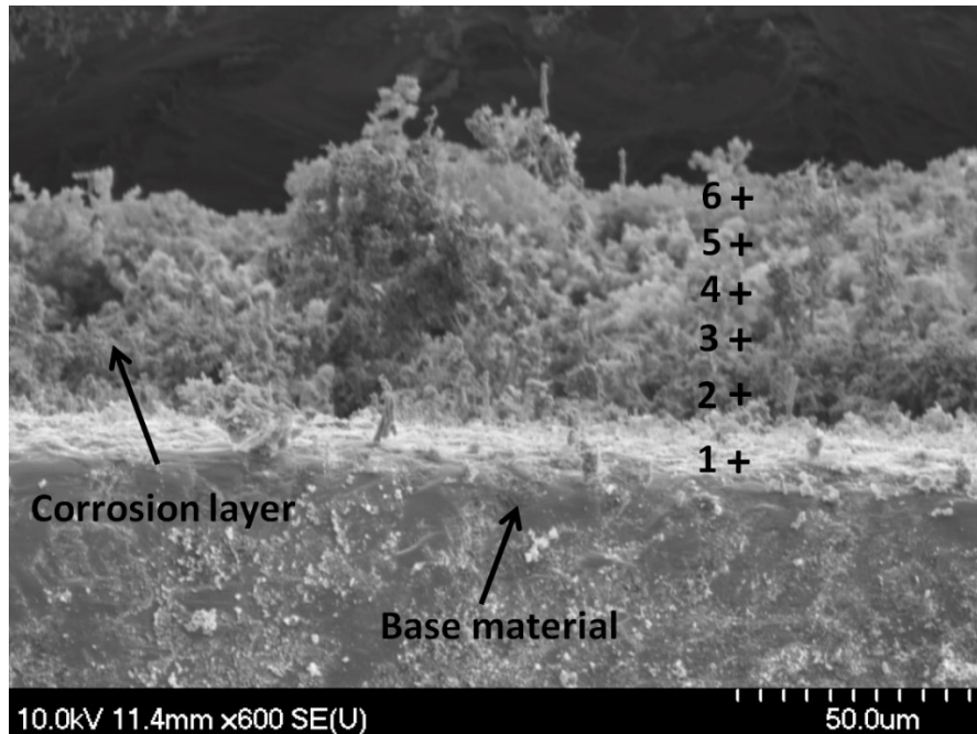
Figure 4-35 EDS (point and ID) analysis on the cross-section of the specimen along the corrosion layer after 185 hours of immersion in the corrosive solution.
