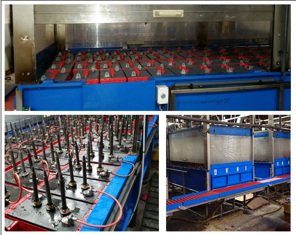
Figure 11 Experimental setup for water-bath formation at SBCL
