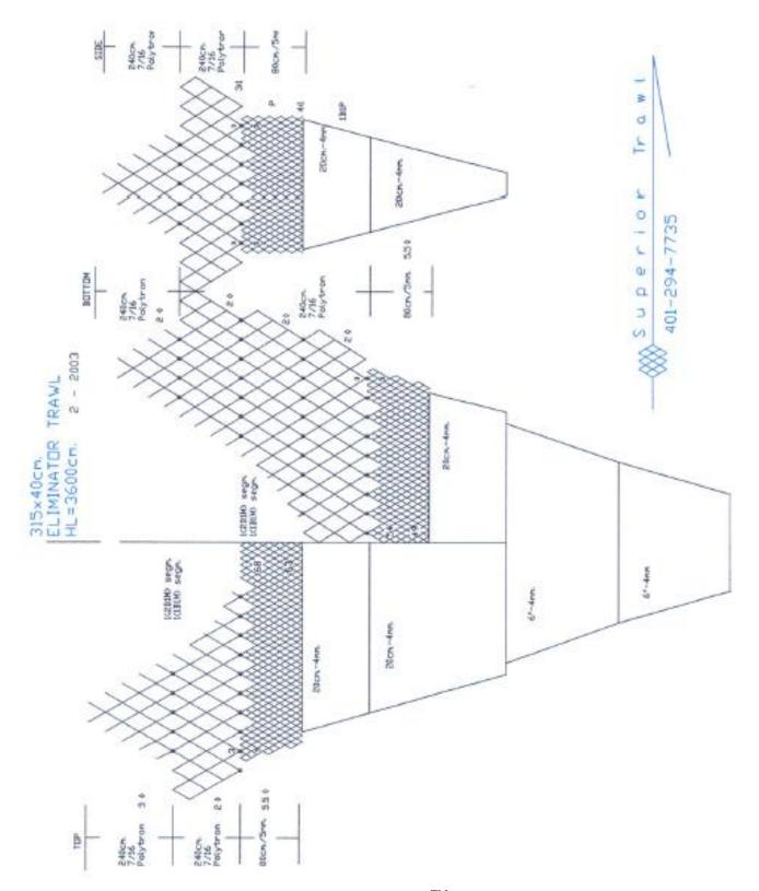
Figure 3 Net design for the Eliminator Trawl<sup>TM</sup> outlining the differences in mesh used in the top and bottom portions of the net, as well as on the wings of the trawl (Beutel et al., 2008).
