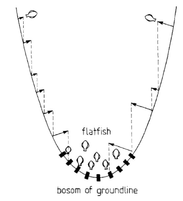
Figure 6 Behaviour of herding flatfish when interacting with groundgear of the trawl (Main and Sangster, 1981).
