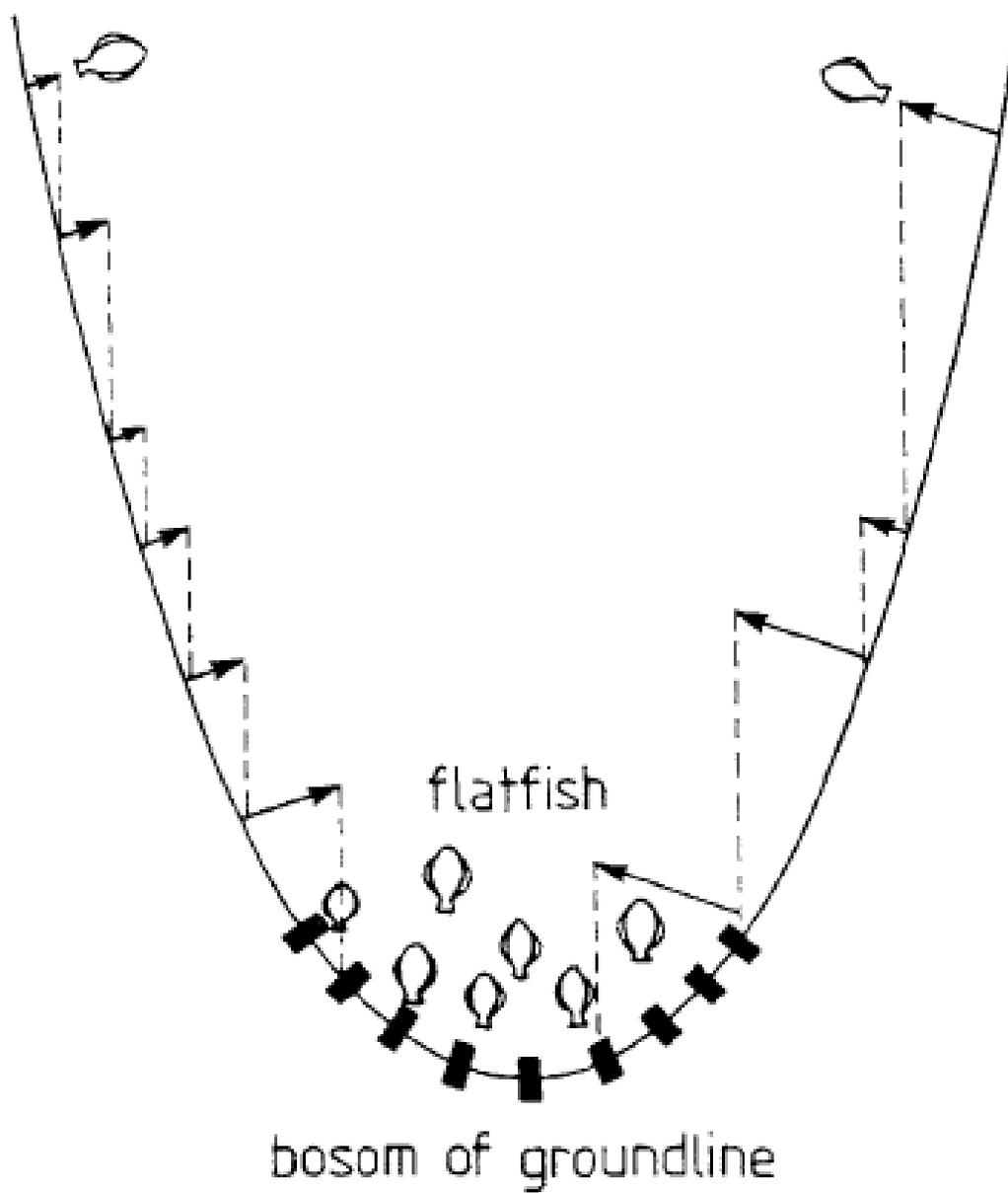
Figure 6 Behaviour of herding flatfish when interacting with groundgear of the trawl (Main and Sangster, 1981).
