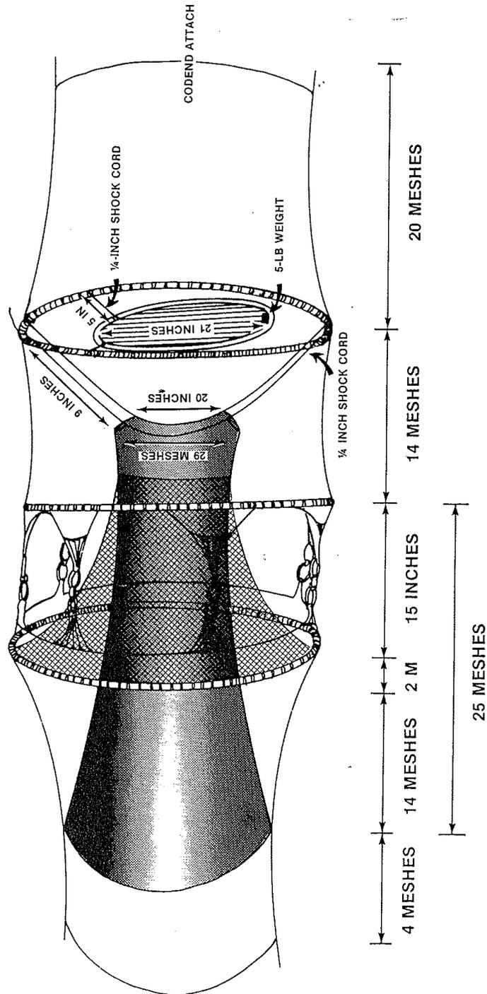
Figure 5 The Finfish separator device, later called the Radial Escape Section. Webbing is removed from the from and middle rings to create an escape opening for larger finfish (Watson et al., 1986)
