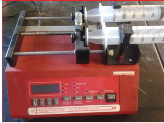
Figure 3.2. Dual syringe Pump from Longer Instruments used to control flow into the mini-fluidic system.
