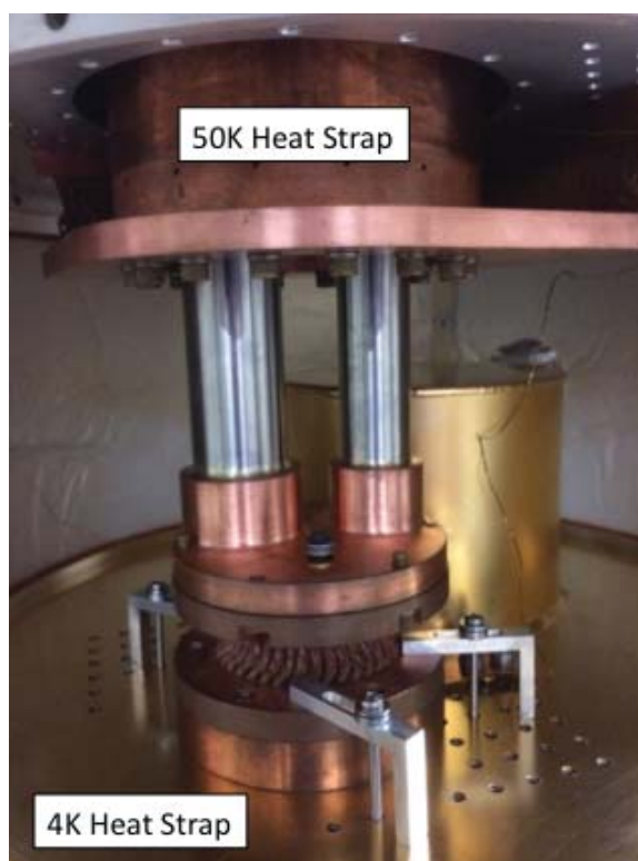
Figure 2.4: 50K and 4K heat straps installed in cryostat.
