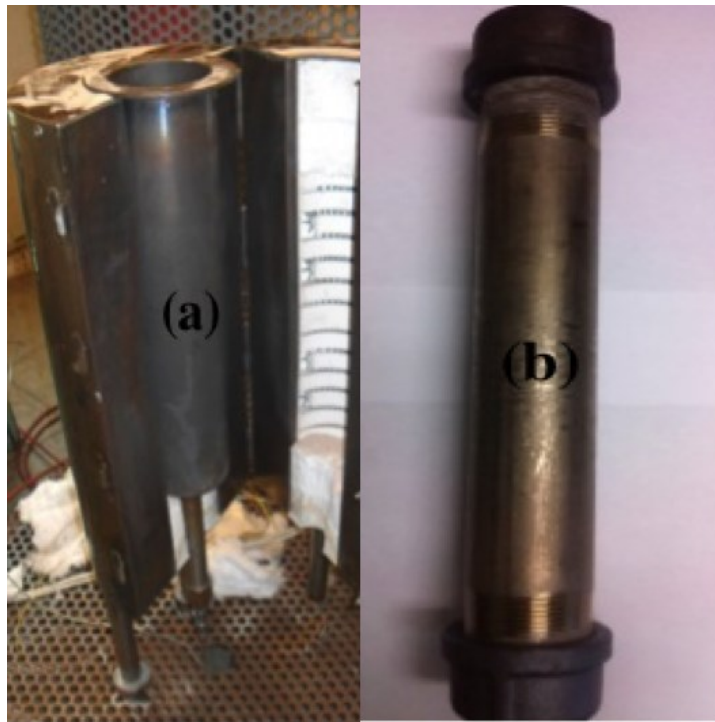
Figure 3- 6: Set up for biomass torrefaction in BFB (a) bubbling fluidized bed reactor (b) reactor tube
