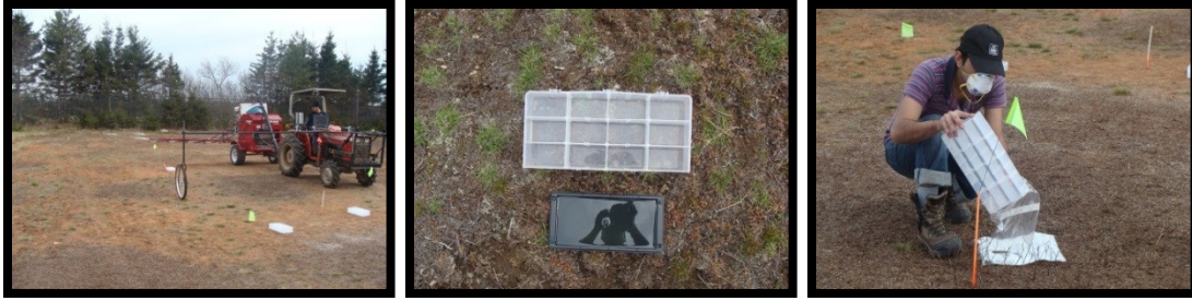
Figure 3-5. Experimental setup for performance evaluation of modified VR spreader in actual wild blueberry field using clay filler.
