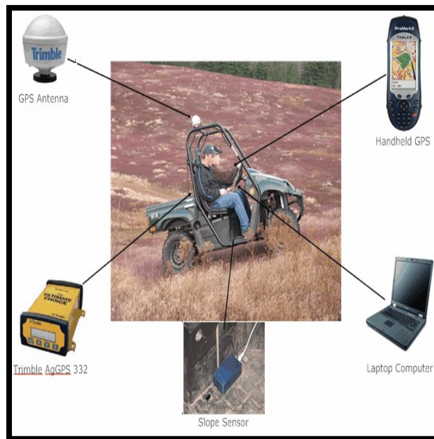
Figure 3-6. Slope Measuring and Mapping System (Zaman et al., 2010a).
