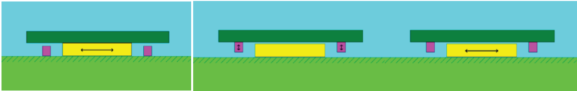
Figure 13. The Floating Platform can be either coupled or decoupled from the XY Pad with the Lifter
