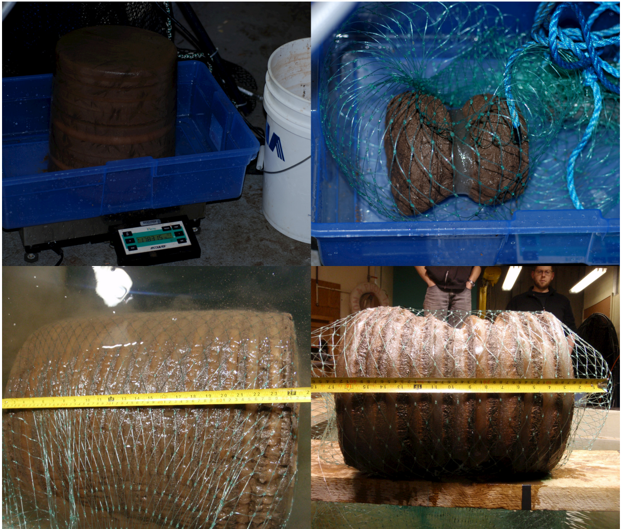
Figure 6.8: Fine grained sediment-laden ice melt photos, showing reduced melt rate where sediment is present for small ice blocks (top) and more uniform melting for large ice blocks (bottom).
