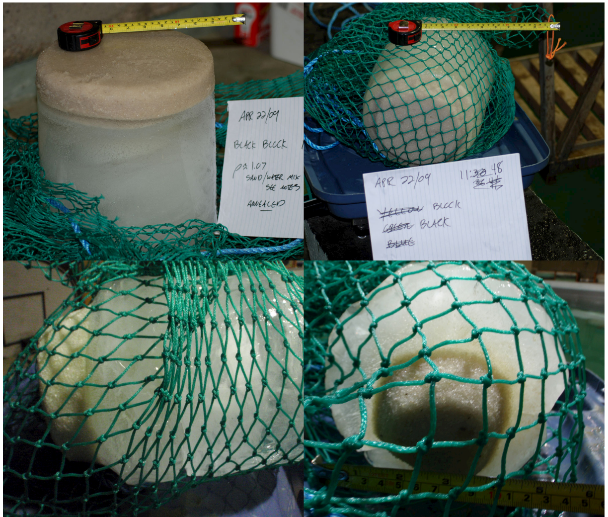
Figure 6.7: Sandy sediment-laden ice melt photos, showing increased melt rate where sand is present.
