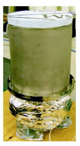
FIG. 5. The radiation shield installed on the cryostat. Liquid nitrogen is filled at the top (after the styrofoam top is removed). The vacuum chamber containing the samples can be seen near the bottom of the picture.
