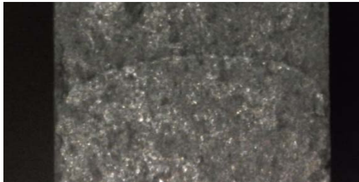
Figure 6.8 Overload marking line on fractured surface
