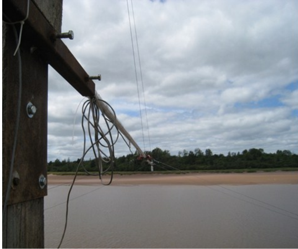
Figure 2.5: Alton Gas Site on the Shubenacadie River, facing west showing the sonar device (Campbell Scientific sonic ranger SR50), suspended 10 m over the river to measure water height.
