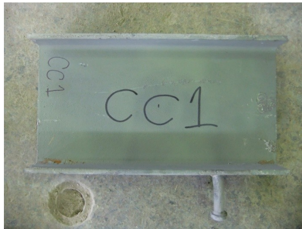
Figure 4.16 Stud deformation of Specimen S1-24-1 after testing
