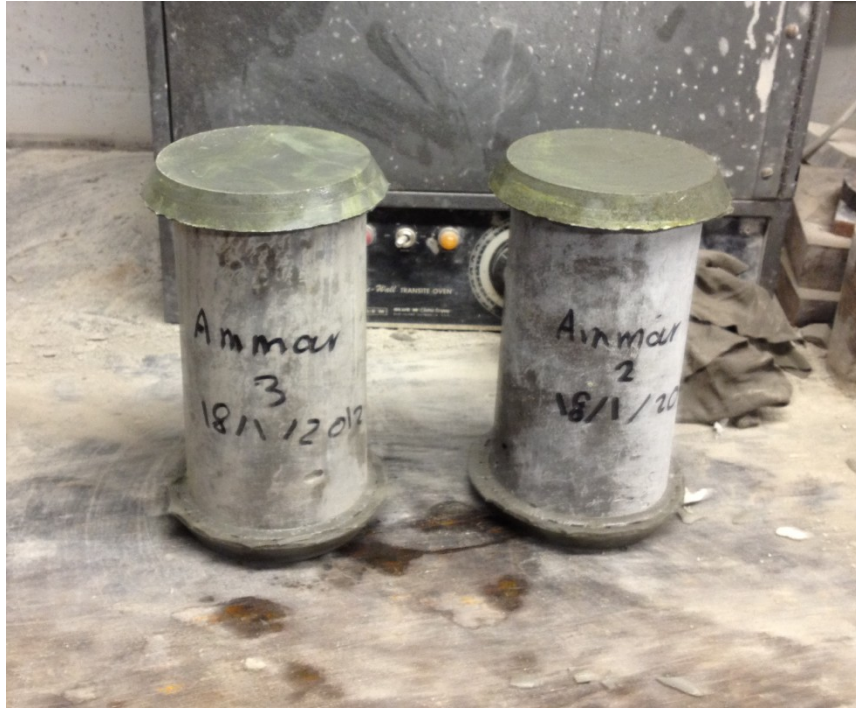
Figure 3.13 Capped concrete cylinders
