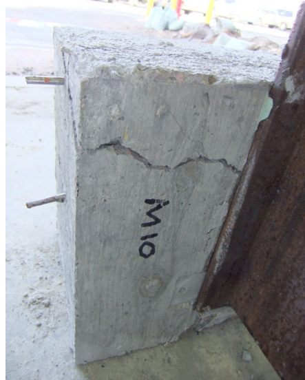
Figure 4.12 Specimen S1-10 after testing
