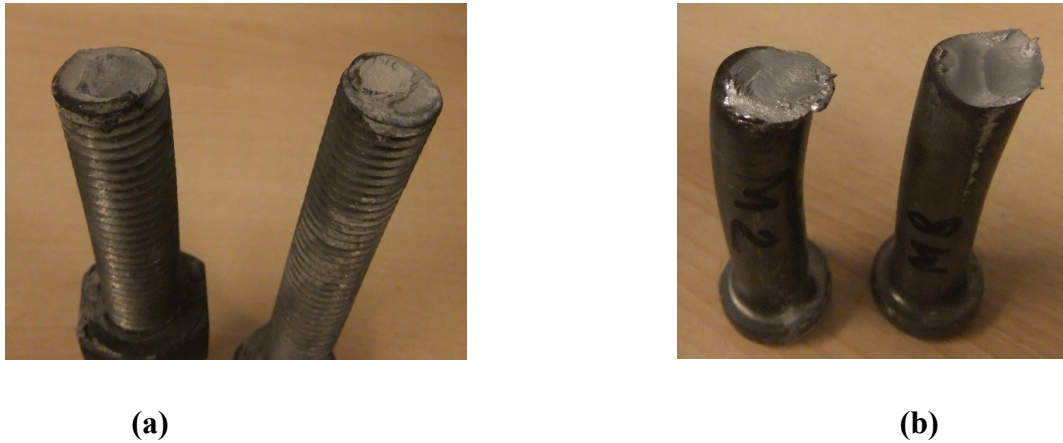
Figure 4.33 Shear studs failure surfaces (a) Adjustable studs, (b) Conventional studs
