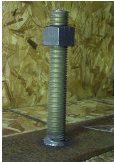
Figure 2.3 Proposed adjustable stud system
