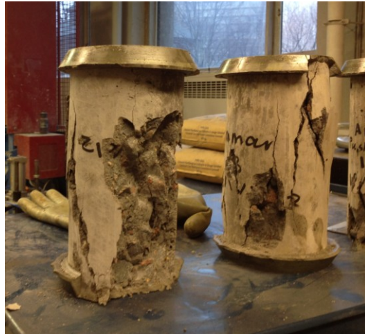
Figure 4.38 Tested concrete cylinders
