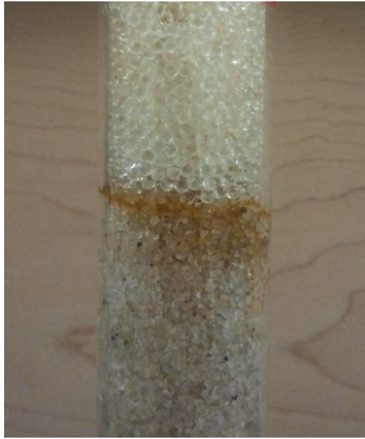
Figure 10: Brownish-orange precipitates an inactive filter
