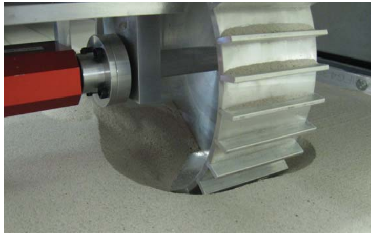
Figure 6.8: Rigid wheel with 32, 10mm grousers operating at a slip ratio of 0.60
