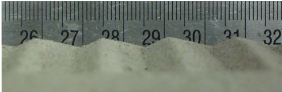
Figure 1.4: Track of a grouser wheel operating in loose sandy soil at a slip ratio of 0.25
