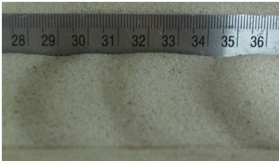
Figure 1.1: Track of a smooth wheel operating in loose sandy soil at a slip ratio of 0.25 with a 48N normal load
