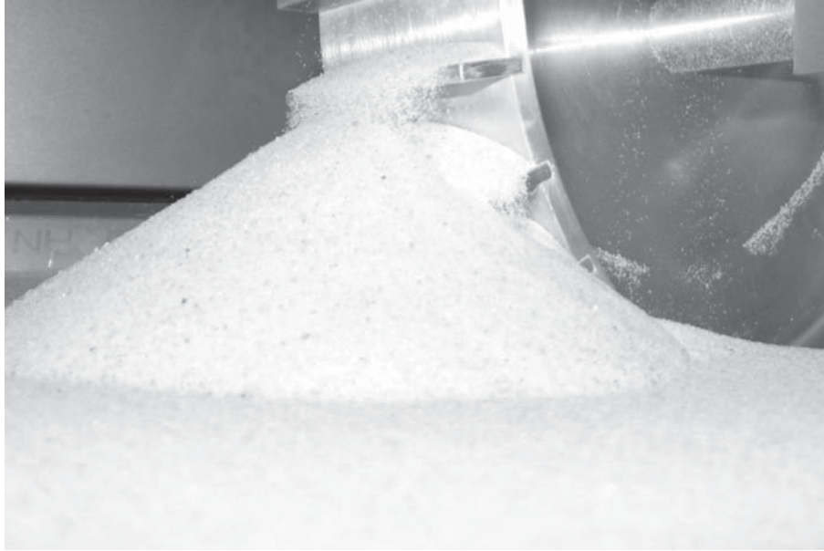
Figure 2.11: Rear prospective view of a rigid grouser wheel operating in sandy soil
