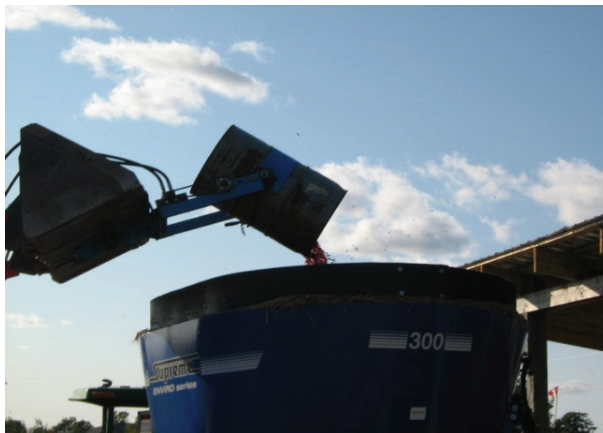
Figure 2.4 Loading SRM into grinder.
