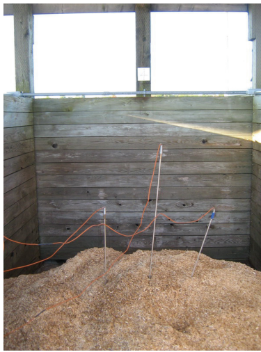
Figure 2.5 Measurement of temperature at three depths in compost pile.
