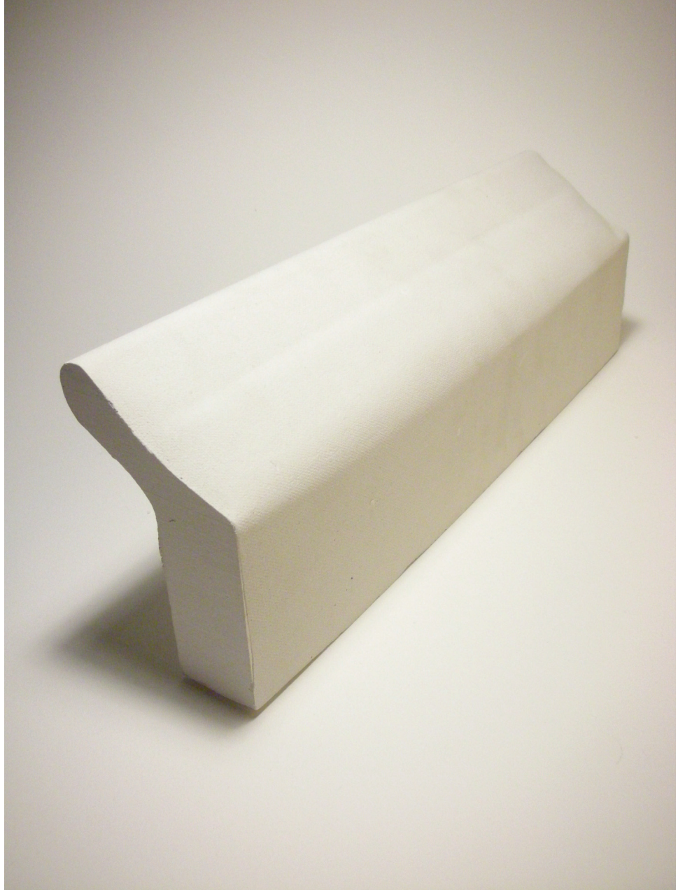
A handrail made by means of fabric formed plaster. It is an extrusion of an earlier sectional study.
